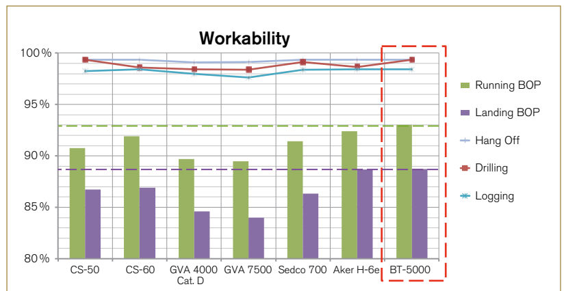
Workability comparison (percent yearly availability due to motions within specified limits) for the BT-5000 MWS and a number of competing designs for operations at a typical North Sea field and limiting motions criteria from a major oil company.
