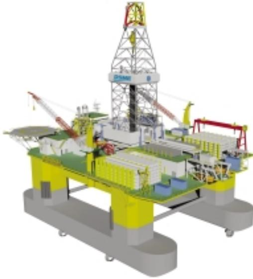
Within its compact arrangement, DSME-6000M facilitates maximum flexibility with regard to various drilling operations through accommodating different drilling facilities, equipment and layouts. Additionally, it possesses dedicated riser storage and spacious pipe racks located on the upper aft deck.
