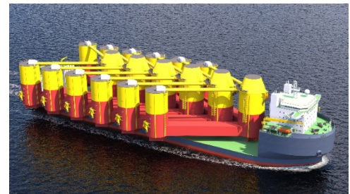
Transport of six 17 MW D-Floaters
